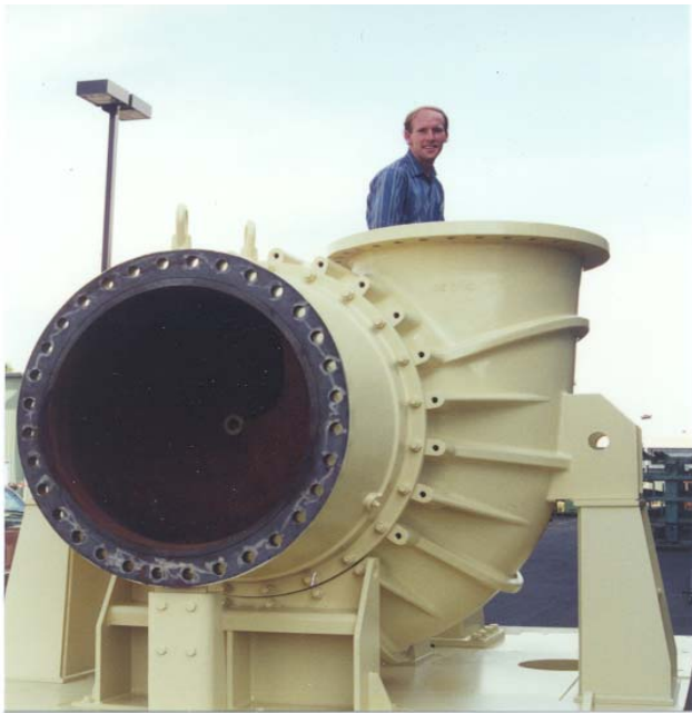
FIG 7a 36" (900mm) Fish Friendly pump installed at Red Bluff, California Duty 2850 l/s @ 7m
