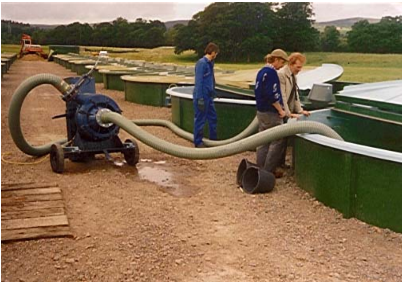
FIG 10b Hidrostat Fish Pump in use on a Hatchery Raising Smolts in Scotland
