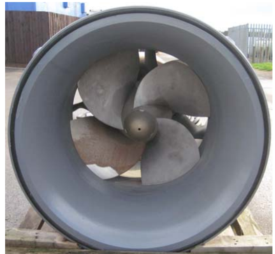
FIG 5a View into Suction showing Axial Flow Impeller
