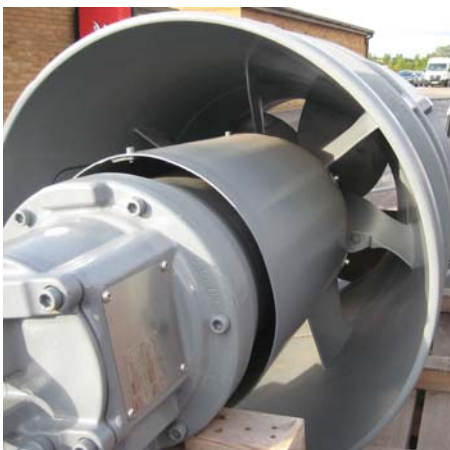
FIG 5b View into Guide Vane Casing showing the Guide Vanes behind the Impeller
